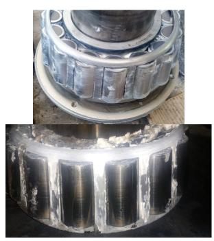
Bearings Using Competitor (Matrix) Grease (after 10 Days)
